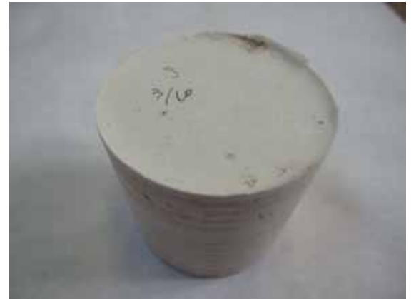
Fig. 1. Articles are cast in separate plaster cylinders
